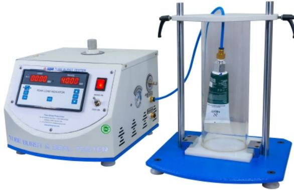
The **Tube Burst Tester** checks the pressure level at which a tube bursts. It can test metal, plastic, rubber, and composite tubes. The tester applies air pressure inside the tube and records the breaking point. The bright LED screen shows clear readings. The machine suits daily quality checks in industries where pressure safety matters. Simple controls and strong clamps make testing smooth. It helps teams to understand tube strength before real use begins.
